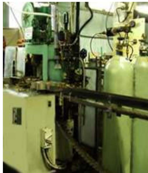
Fig. 3: Bottling line and CO<sub>2</sub> for carbonisation of soft drinks.
